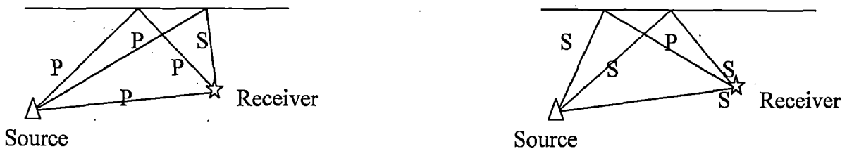
Figure 2.3: Free surface effect.
