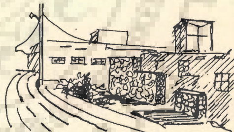
Fig. 3.109 : Coral Stone Used for Building Construction, District 1 - B'Lengeh
