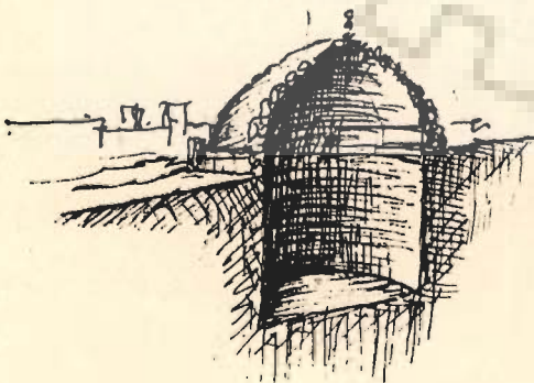
Fig.1.32 : "Berkeh" built with Coral Stone and Lime Concrete
