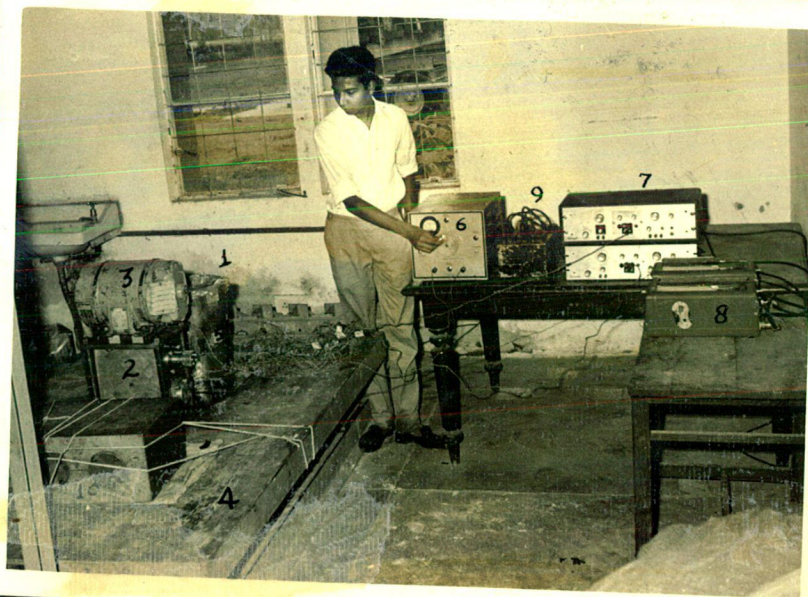
Fig. 4.4 Arrangement for Steady State Vibrations.
