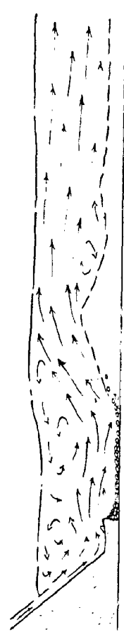
C. TAILWATER ABOVE MAXIMUM. FLOW DIVING FROM APRON SCOURS CHANNEL.
