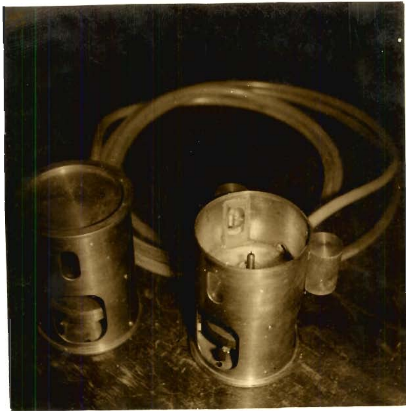
FIG. 2-7. PHOTOGRAPH OF THE PORTABLE WATER TUBE TILTMETER SYSTEM IN ITS INITIAL STAGE OF DEVELOPMENT
