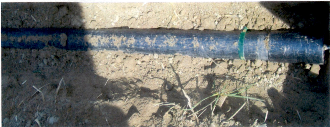
Fig.3.3 A MFS06 magnetic induction coil in the parallel testing survey
