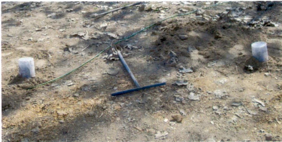
Fig.3.6 Two buried vertical magnetic sensors in parallel test site
