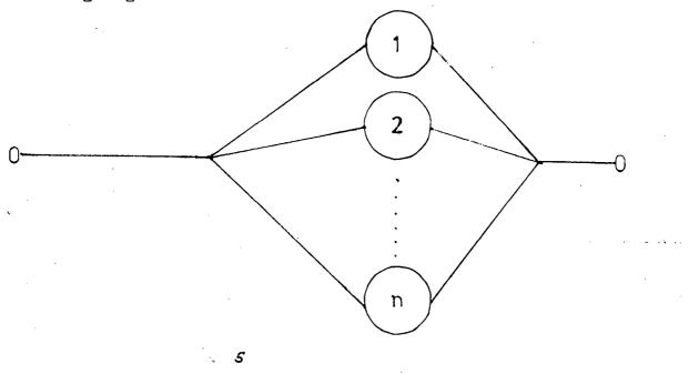
In this case the system can function properly when at least one of the components is working i. e. the system fails only when all the components fail. The reliability of a parallel system consisting of n units is given as
