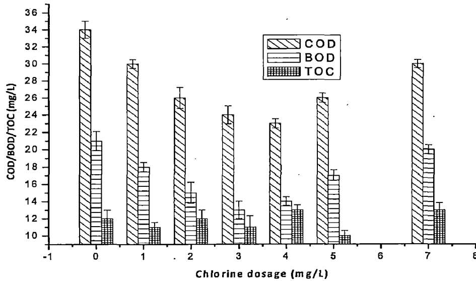
Fig 3.3.4c. COD, BOD and TOC variation during chlorination.
