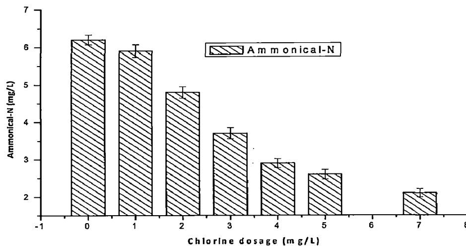
Fig 3.4.10c. Effect of chlorination on ammonical nitrogen
