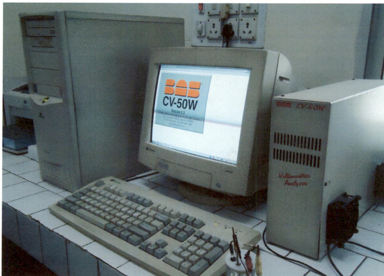
Fig. 1.4 Bioanalytical system used for the electrochemical studies.
