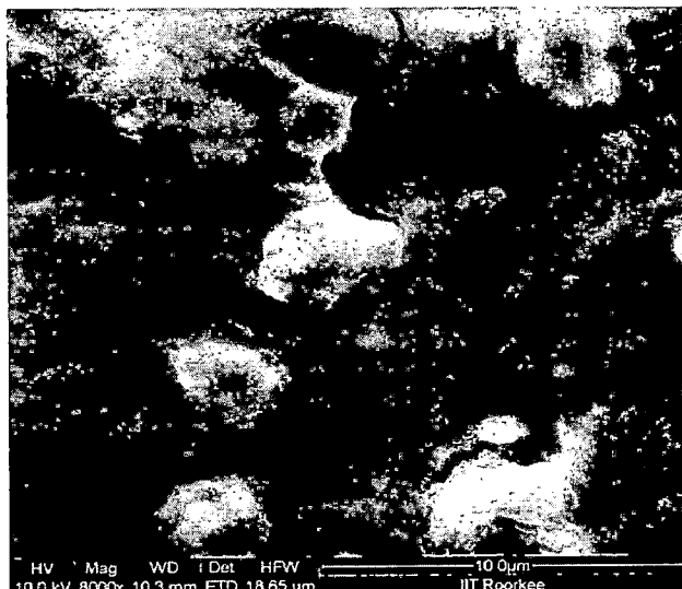
Fig. 2.6a. SEM image showing morphology of MP-0.4 batch synthesized by stirring pectin, MNPs and \text{Ca}^{2+} for 1 h.
