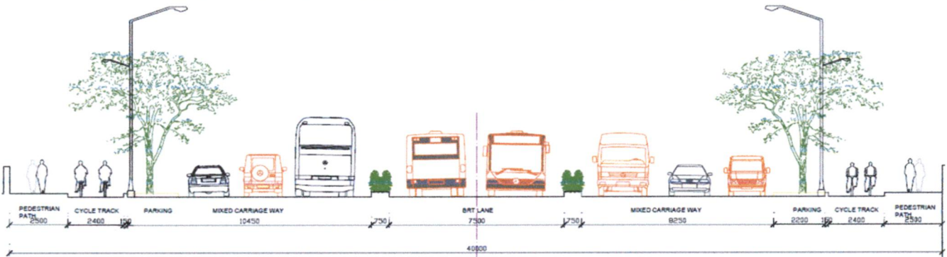
FIGURE 4-3 TYPICAL CROSS SECTION OF 40 M ROW BRT CORRIDOR ROAD
