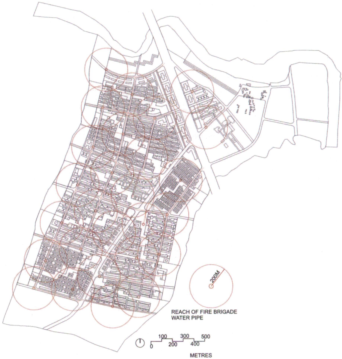
Figure 7-17: Punawale firefighting layout
