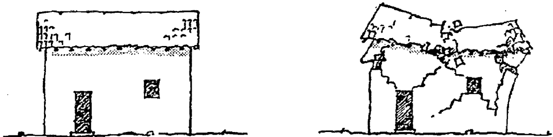
Figure 5.3 Failure in mud walls
