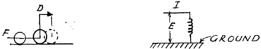
(a) MASS POINT AND ITS ELECTRICAL ANALOGUE .
