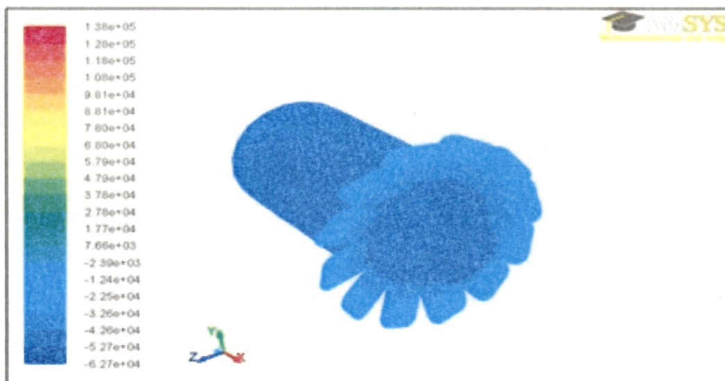
Figure 5.15: Total pressure variation on wicket gate
