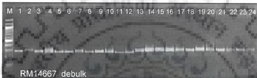
Fig. 4.14 PCR amplification of individual plants constituting the bulk with RM14667; Lane 1: PR106, Lane 2: Basmati 370, Lanes 3-12: -ve debulked lines, Lanes 14-24: +ve debulked lines, M: Molecular weight marker
