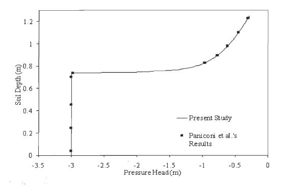
Fig. 3.5: Model validation for infiltration into a dry soil- Neuman boundary condition: Comparison of Pressure heads
