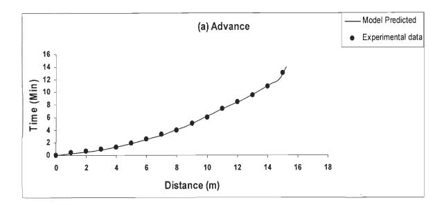
Fig. 5.2 Comparison of model predicted and experimentally observed advance for border strip 1
