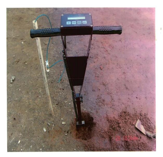
Plate 4.1: Soil Moisture measurements being done using TDR Soil Moisture Meter
