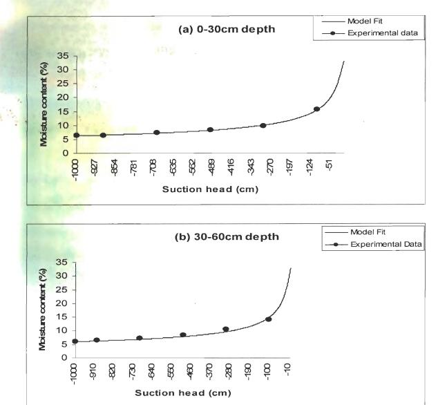
Fig. 4.3: Van Genuchten model fit for soil moisture data at location 1
