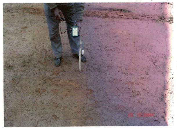
Plate 4.3: Measurement of soil suction head by digital meter in the field
