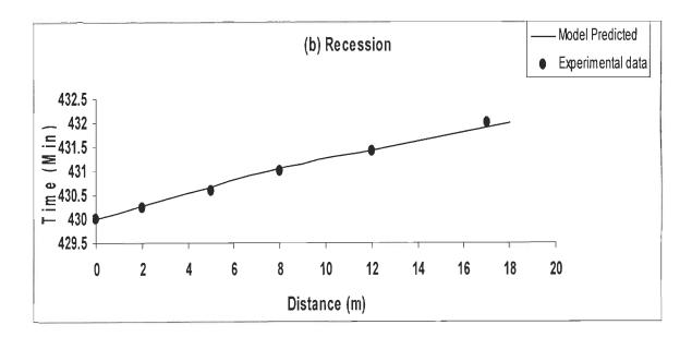
Fig. 4.9: Comparison of model predicted and experimentally observed advance and recession-border strip 2
