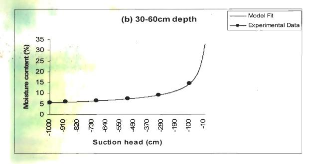
Figs. 4.5: Van Genuchten model fit for soil moisture data at location 3
