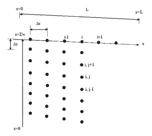
Fig. 3.2: Finite-Difference grid for numerical solution
