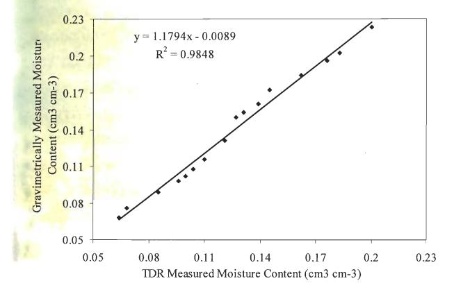
Fig. 4.1: Calibration curve for TDR Soil Moisture Meter
