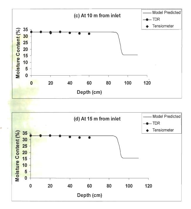
Fig. 4.8: Comparison of model predicted and experimentally observed moisture content-border strip 1
