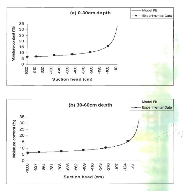
Fig. 4.4: Van Genuchten model fit for soil moisture data at location 2
