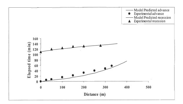
Fig. 3.9: Comparison of model predicted and experimental advance and recession field 3
