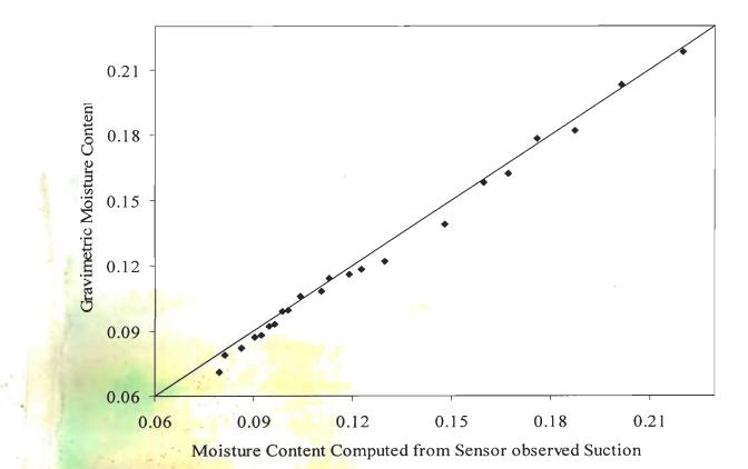
Fig. 4.2: Laboratory and Sensor computed Moisture Content values along 1:1 line.
