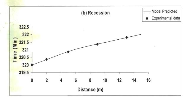
Fig. 4.7: Comparison of model predicted and experimentally observed advance and recession-border strip 1
