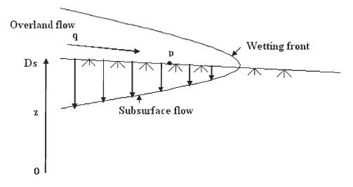
Fig. 3.1: Schematic diagram of border strip irrigation
