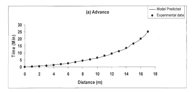
Fig. 5.5 Comparison of model predicted and experimentally observed advance for border strip 2
