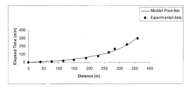
Fig. 3.7: Comparison of model predicted and experimental advance for field 1
