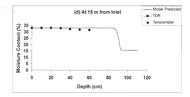
Fig. 5.4 Comparison of model predicted and experimentally observed moisture content profile for border strip 1
