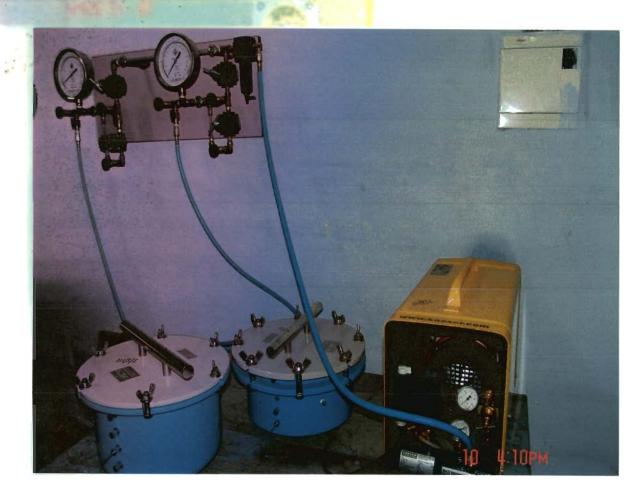
Plate 4.5: Pressure Plate Extractor
