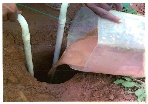
Plate 4.2: Soil Moisture Sensor installation in the field
