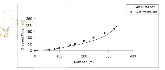
Fig. 3.8: Comparison of model predicted and experimental advance for field 2
