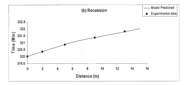
Fig. 5.3 Comparison of model predicted and experimentally observed recession for border strip 1
