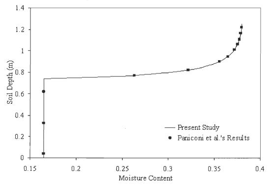
Fig. 3.6: Model validation for infiltration into a dry soil- Neuman boundary condition: Comparison of moisture content
