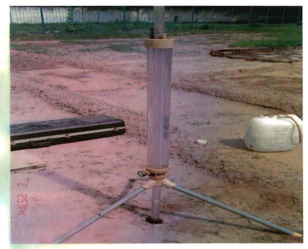
Plate 4.4: Measurement of Saturated Hydraulic Conductivity in the field using Guelph permeameter
