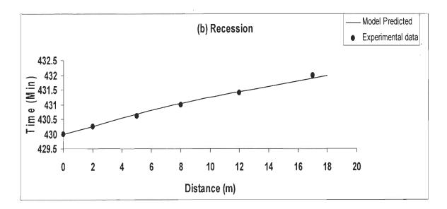
Fig. 5.6 Comparison of model predicted and experimentally observed recession for border strip 2
