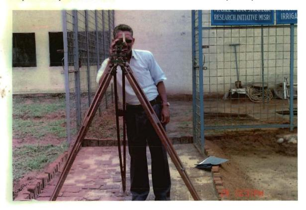
Plate 4.7: Set up of Dumpy level during experiment
