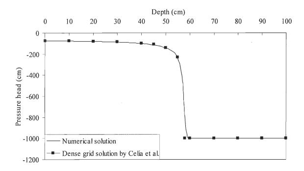
Fig. 3.3: Model validation for infiltration into a very dry soil: Dirichlet boundary condition at top
