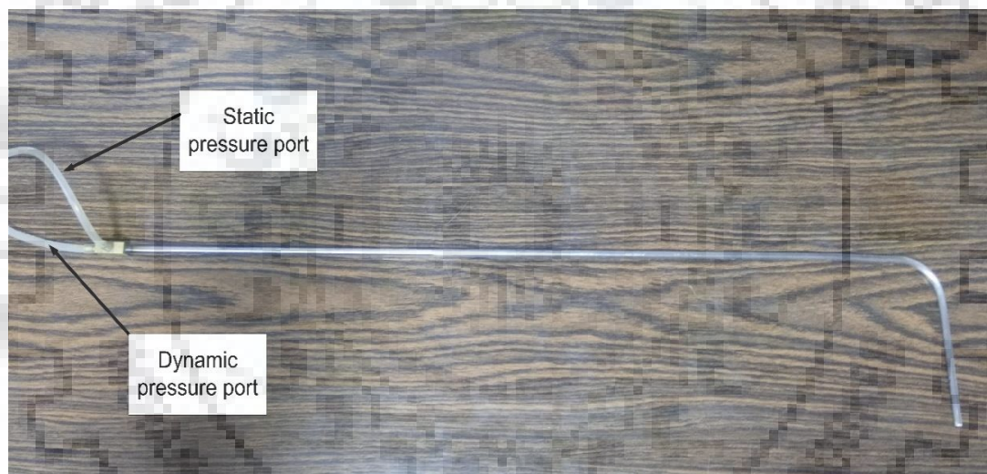
Fig. 4.5 Pitot tube for calibration of velocity measured from hotwire anemometer.
