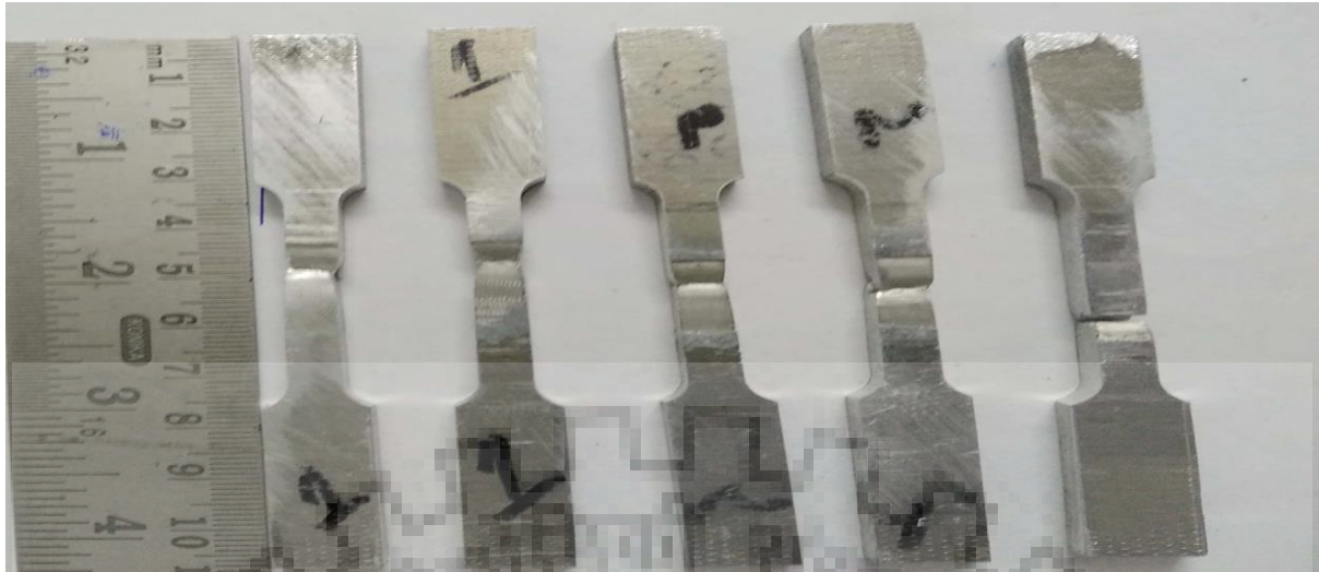
Fig.13: Tensile Test Specimen after failure
