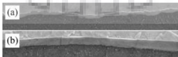
Fig. 11 Microstructures (SEM) of joint at central region of galvanised steel/aluminium alloy interface at different welding currents (Zhang et al., 2011) [10].
