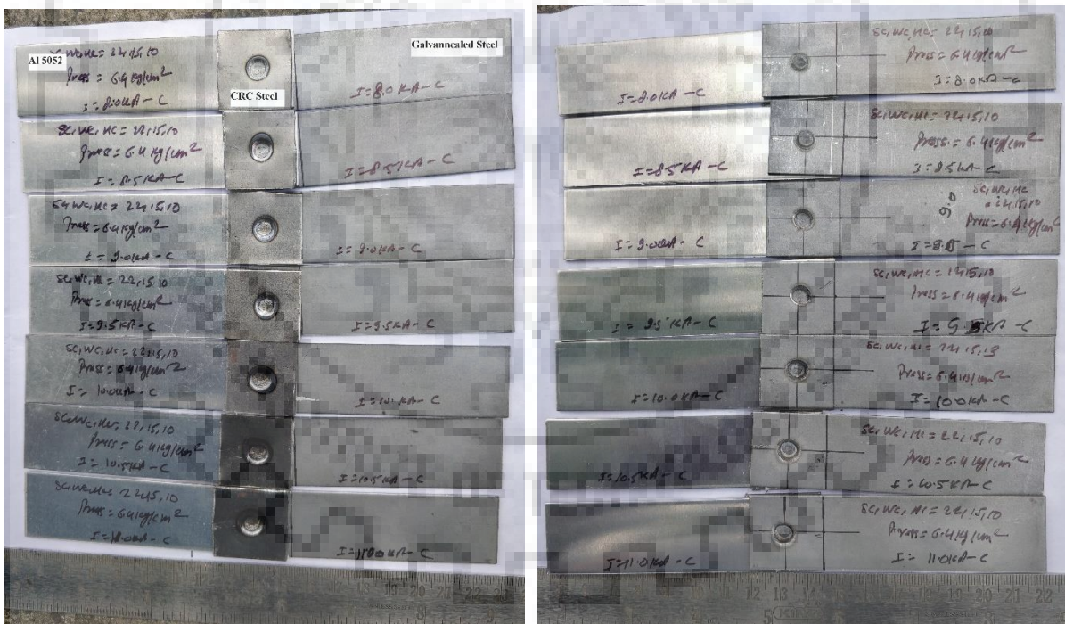
Fig. 28 Actual welded sample for joint with cover plate at welding current 8.0 kA to 11.0 kA with an increment of 0.5 kA.
