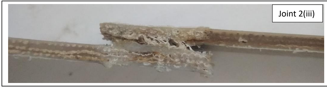
Fig.21 Fracture of Type 2 lap joints configuration of composite
