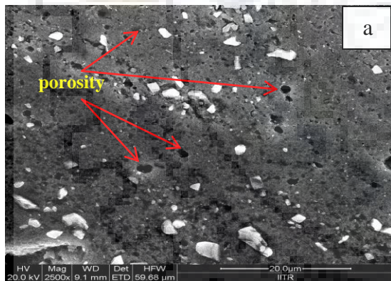
Fig. 5.12: FSPed specimen Shows distribution features of SiCp in stir zone (SZ) at FSP parameters of 708 rpm and 40mm/min (a) SEM image of AA7075/SiCp composite, (b) weight (%) of Si (c) EDX indicates percentage of Si in SiCp enrichment region.
