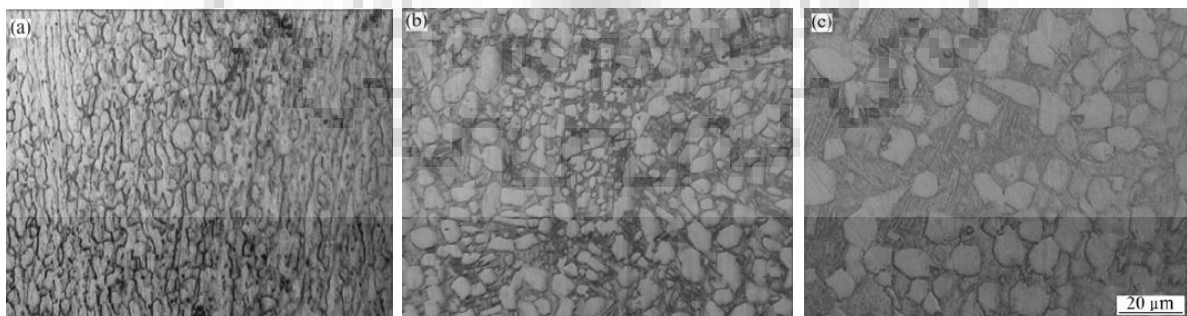
Fig. 12: Globularization (at 920°C, 2hours) post hot rolling at temperatures (a) 820°C (b) 870°C (c) 920°C [18]
