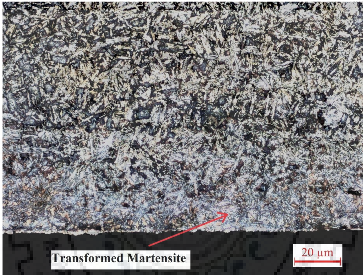
Figure 4.8: Optical micrographs of cross-section of the pin sample after wear
