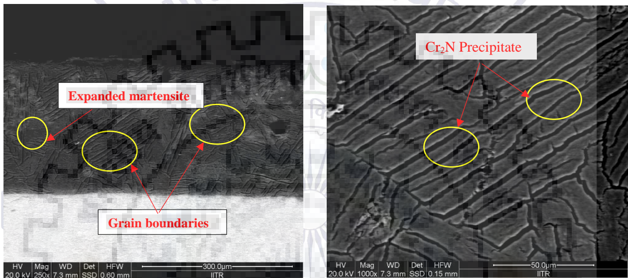
Fig (27a) back scatter image showing Grain boundary
