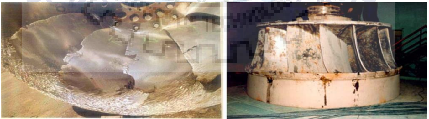
Fig. (1) Runner blades showing cavitation erosive failure [1]
