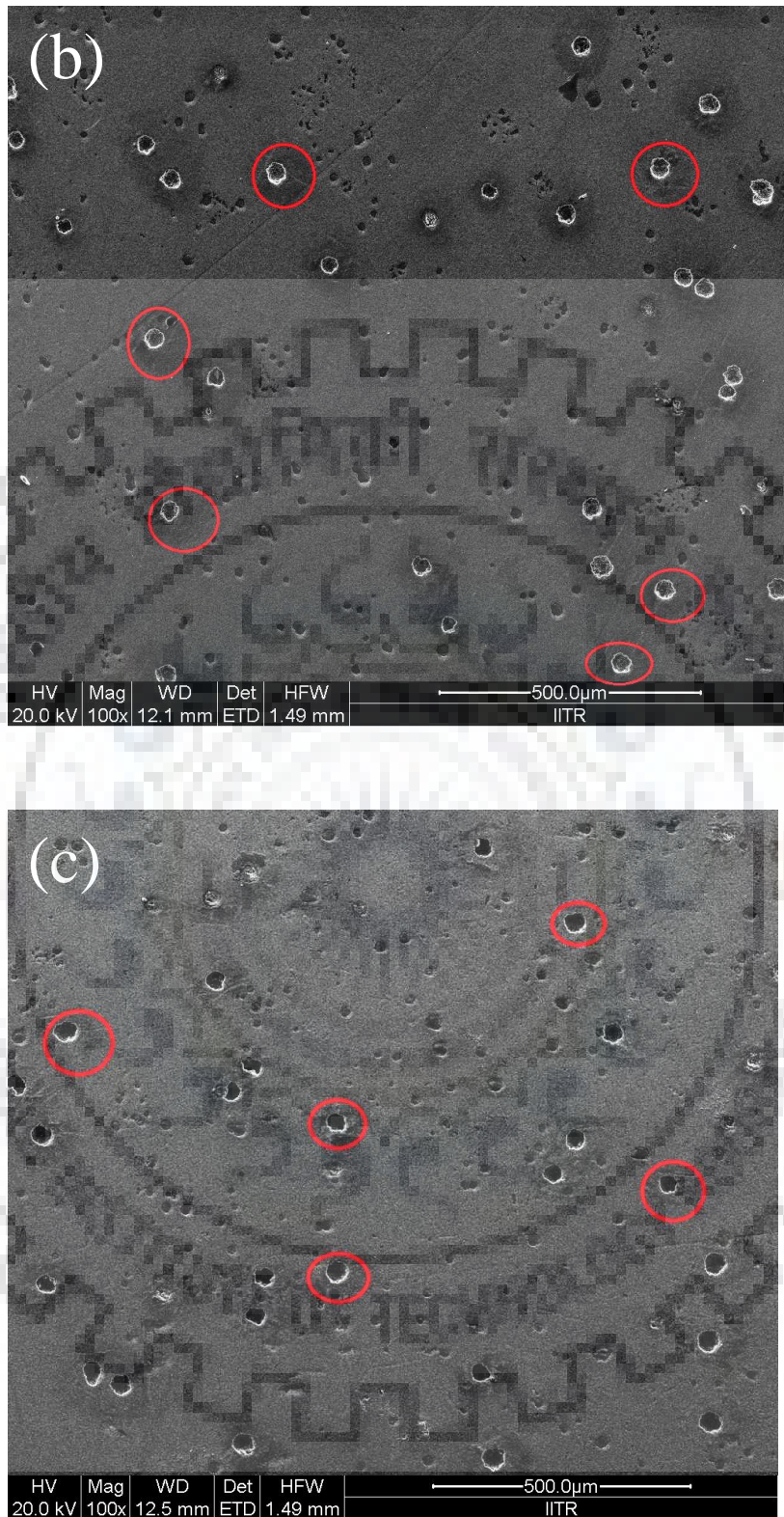
Fig 19: SEM image of the surface of the samples after erosion testing of (a) 12 hour 90° impact angle (b) 6 hour at 75° impact angle (c) 6 hour at 90° impact angle
