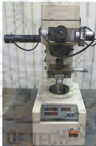
Fig. 3.5(a). Leco LV 700 Vickers hardness tester
