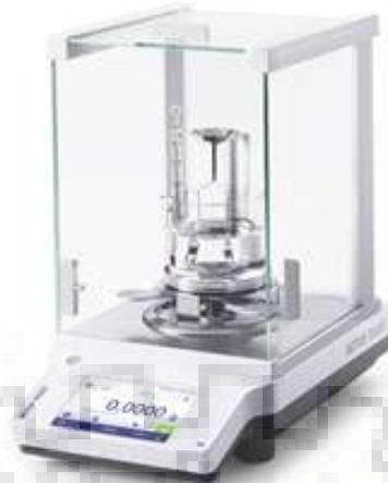
Fig. 14 Mettler Toledo weighing machine with density kit setup
