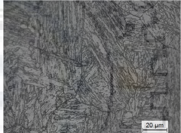
b ) 950°C-2 hr-OQ-600°C-1 hr MSS at 100X
