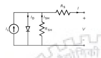
To understand the electronic behavior of a solar cell, it is useful to create a model which is electrically equivalent, and is based on discrete electrical components whose behavior is well known.
