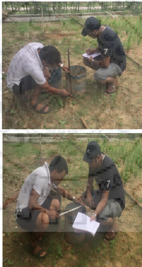
Figure 4. 6 Infiltrometer set up
