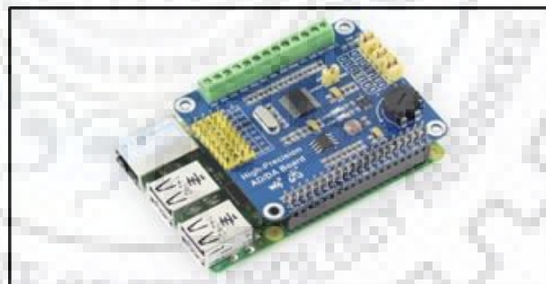
Figure 4.15 ADC module mounted on Raspberry pi processor
