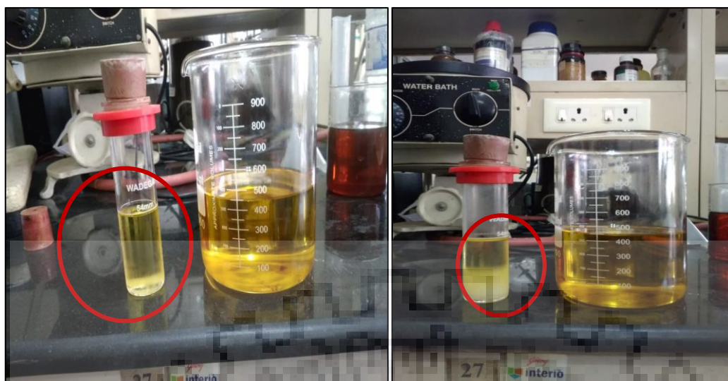
Fig 2.13 Sample showing (a) haze appearance indicating cloud point (b) Solidify state for pour point
