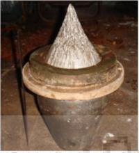
(a) Eroded needle and seat ring of machine unit 1
