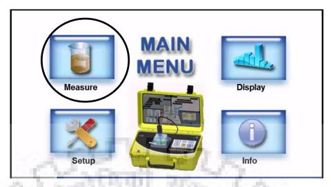
Figure 4.5: Main menu screen of LISST- Portable particle size analyzer
