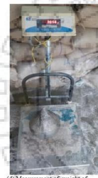
(d) Measurement of weight of eroded spear on electronic weigh scale
