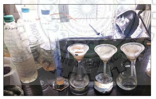
Figure 4.15: Experimental set up for performing gravimetric analysis
