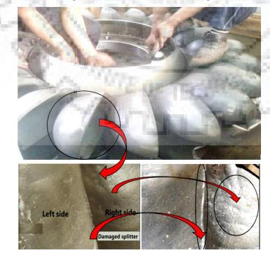
Figure 4.31: Images of Runner and eroded buckets of Pelton turbine of CHEP-I.
