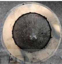
(b) Visible Gap between spear and seat ring due to erosion
