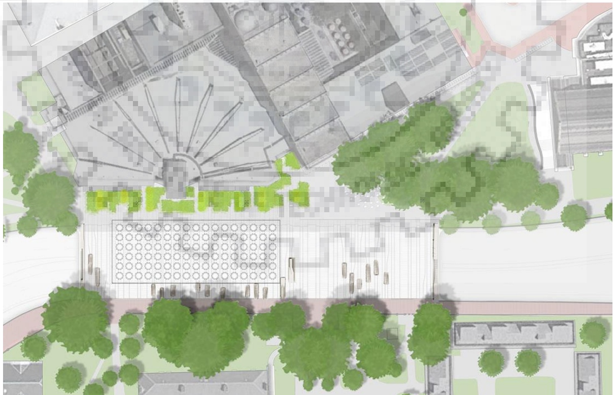
Figure 21 - Plan of the plaza showing layout of the benches.
