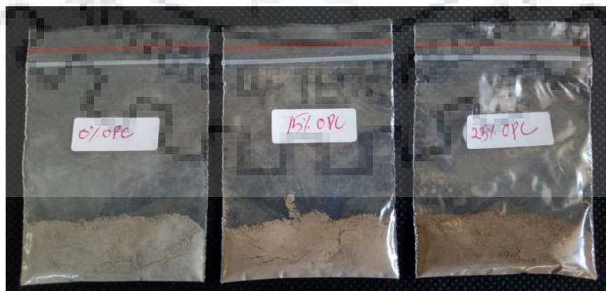
Figure 7: Samples of OPC with jarosite compositions of 0%, 15% and 25% for XRD analysis
