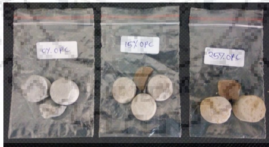
Figure 4: Dry pellets of OPC with jarosite compositions of 0%, 15% and 25% before grinding
