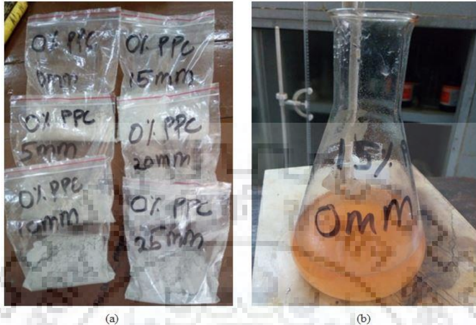
Figure 26: (a) Samples obtained from a specimen of 0% PPC. (b) One of the samples after reaching the titration endpoint.
