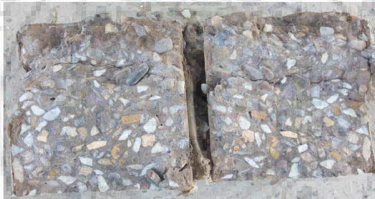
Figure 15: One of the specimens split into two at the end of the test period
