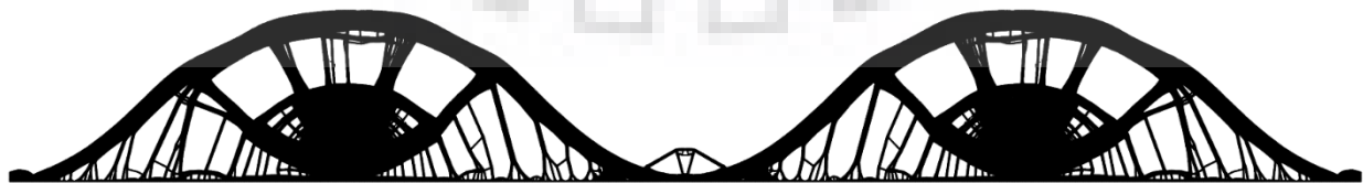
Fig 5.13: Bridge form obtained for volume fraction of 0.13.
