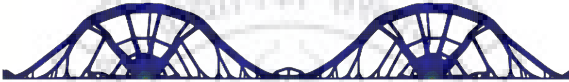
Fig 5.14: Bridge form obtained for volume fraction of 0.13 with a mesh size of 5 m. Same form is obtained for a non-linear analysis.
