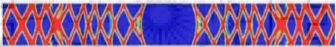
Fig. 2. 5 Symmetry constrained optimisation study on 5 m span UB 305* 165*40 with volume fraction of 0.4 ( K.D Tsavdaridis et al ,2015)
