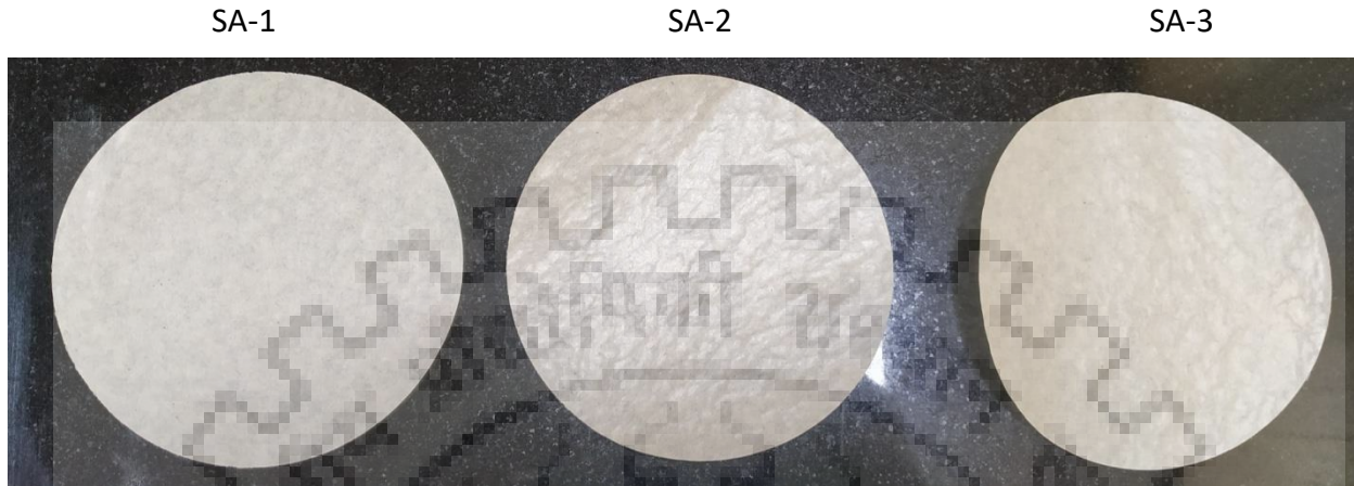
Figure 11: Coated sample of sodium alginate based coating.
