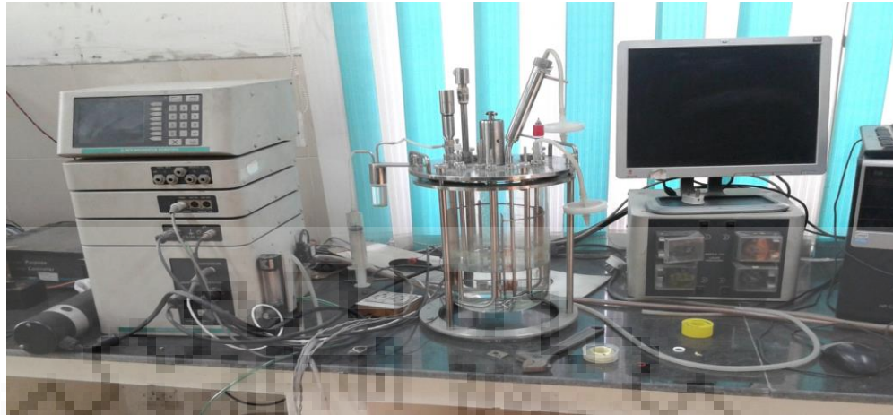
Figure 3.2a Experimental Setup of 7.5 L Stirred Tank Bioreactor
