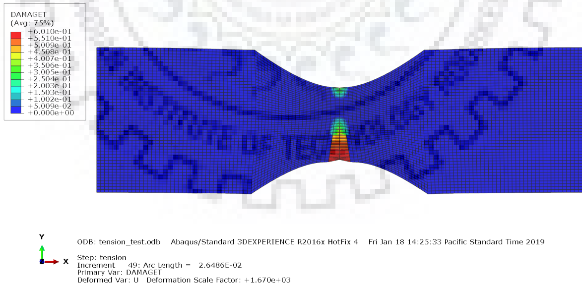
Figure 8.18: Localized crack propagation in the bar
