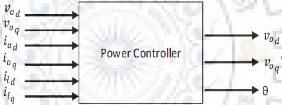
Figure 4. 3: Power controller block having input and outputs in d-q frame in isolated mode.
