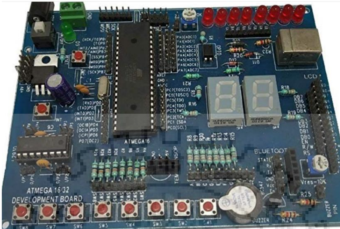
Figure 3. 8 AVR16/32 Development board
