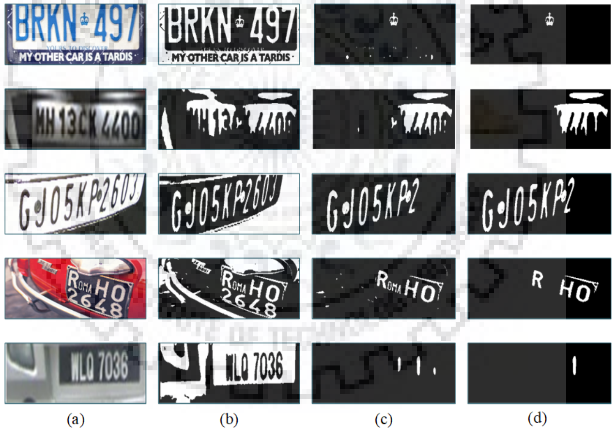
Fig. 4.12. Some typical failure cases of Adaptive CS module. (a) Detected license plate image. (b) Otsu thresholding using Adaptive module. (c) Border thresholding. (d) Final segmented image after removal of low pixel value objects.
