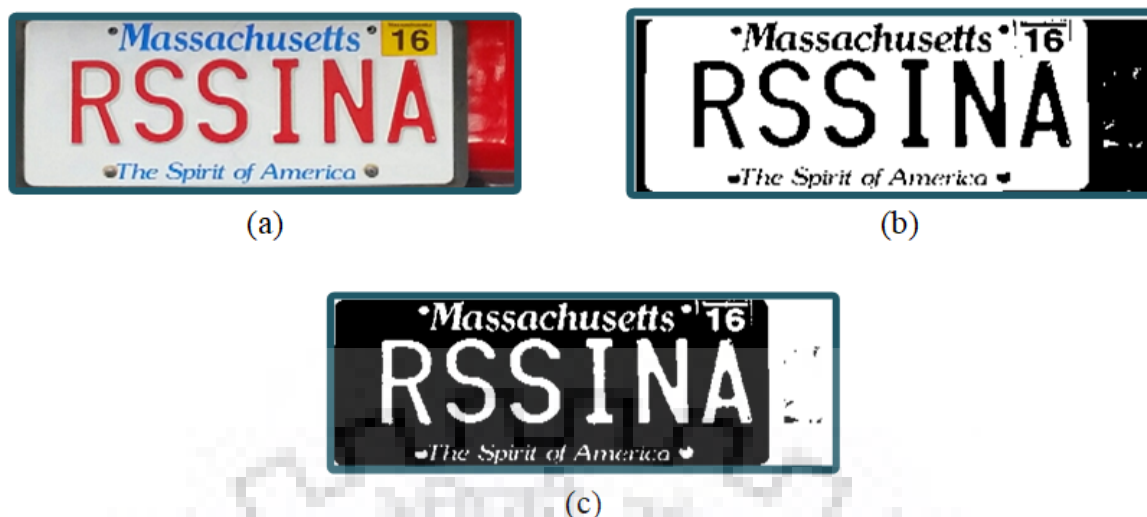
Fig. 3.15. Visualization of binarized output using Otsu thresholding. (a) Detected license plate image. (b) Otsu thresholded image. (c) Correct binarized image derived from adaptive module.
