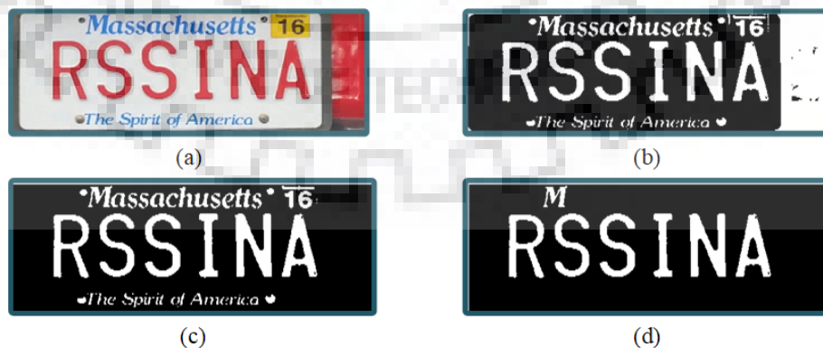
Fig. 3.17. Removal of Objects of low pixel value. (a) Detected license plate image. (b) Correctly binarized image using adaptive module. (c) Border thresholded image. (d) Low pixel value objects removal.
