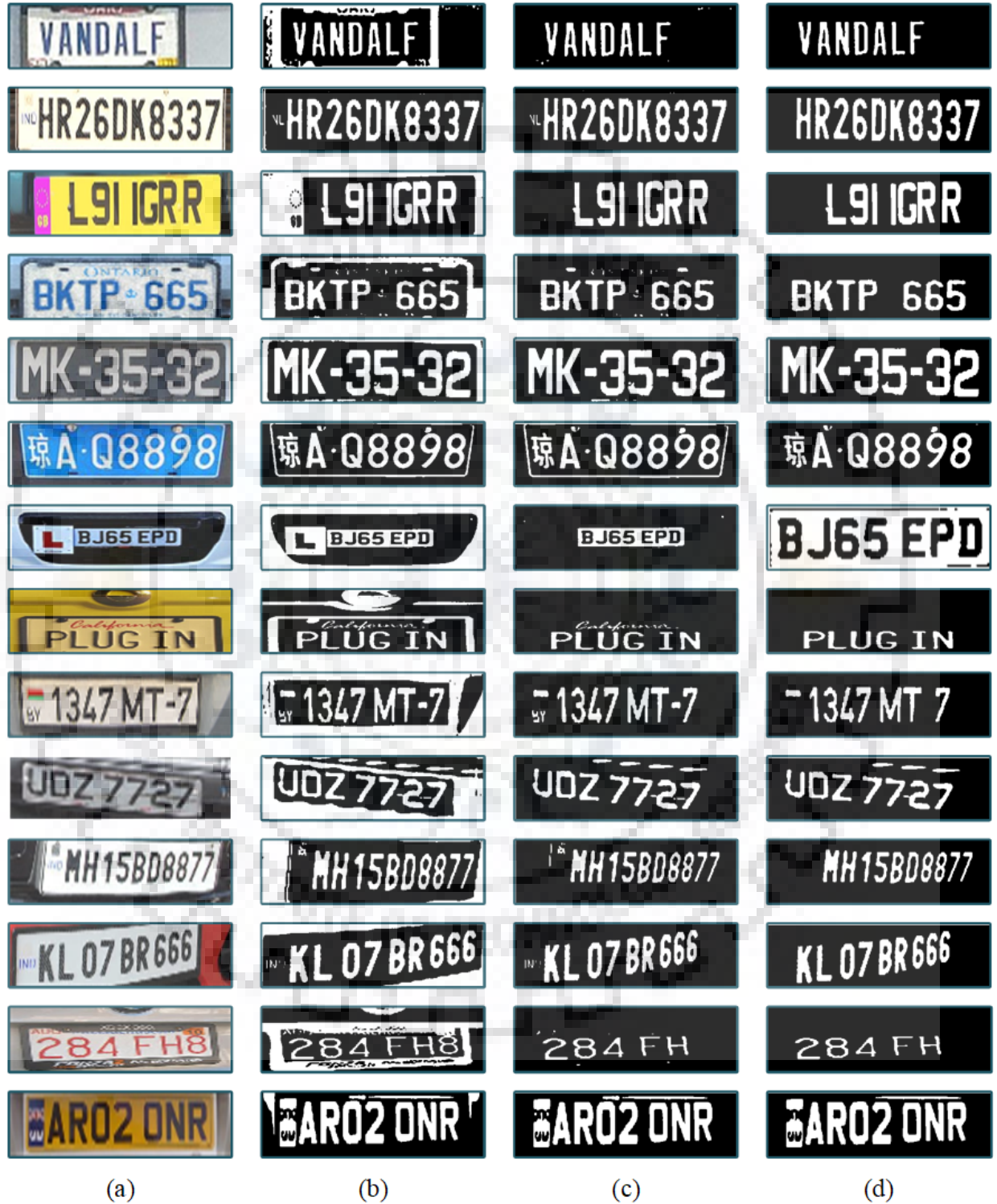
Fig. 4.3. Visual Results of Adaptive CS Module. (a) Detected license plate images. (b) Binarization using Otsu thresholding and adaptive module. (c) Result of Border thresholding. (d) Final segmented characters after removal of low pixel objects.
