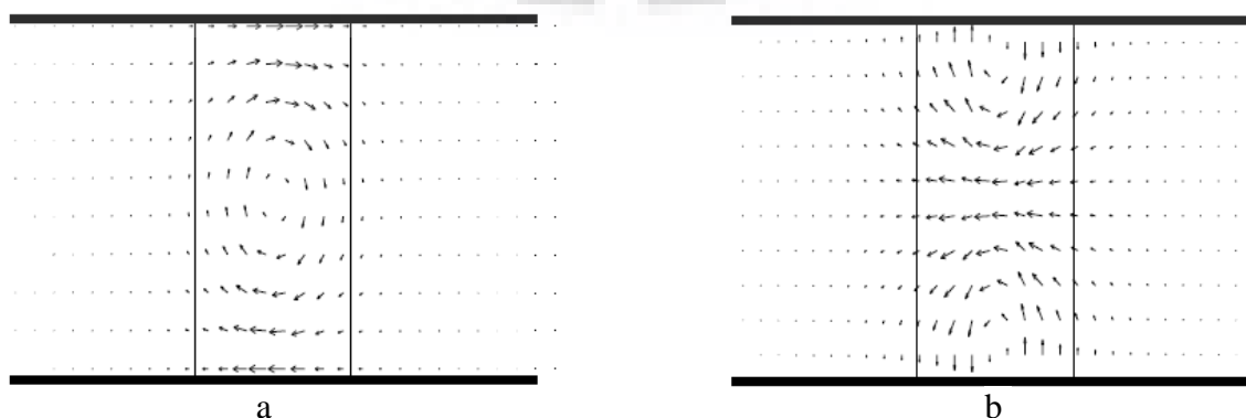
Fig. 1.2 (a) LSE 11 Mode, Magnetic Field & (b) LSM 11 Mode, Electric Field
