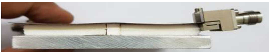
Fig. 5.16 Gap in Foam-PLA & Foam-Base Plate
