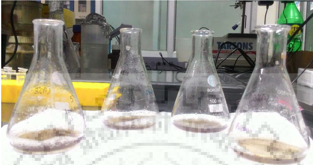
Fig. 5.7.2 Sample preparation step of 3% and 4% acid pretreated samples in the flasks for HPLC
