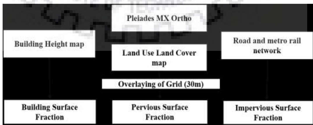
Figure 4-7: Methodology for computation of surface cover fraction
