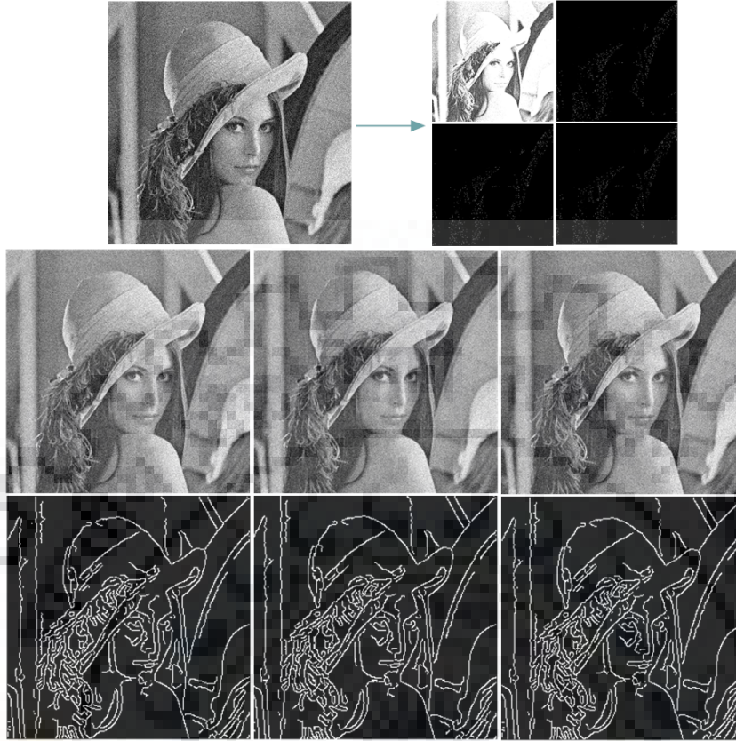
Figure 5.1: The first row shows the image decomposition using wavelet transform into A , H , V , D parts; The second row shows the reconstructed detail parts I_H , I_V and I_D ; The third row shows the edge details of images I_H , I_V and I_D using Canny edge detector.
