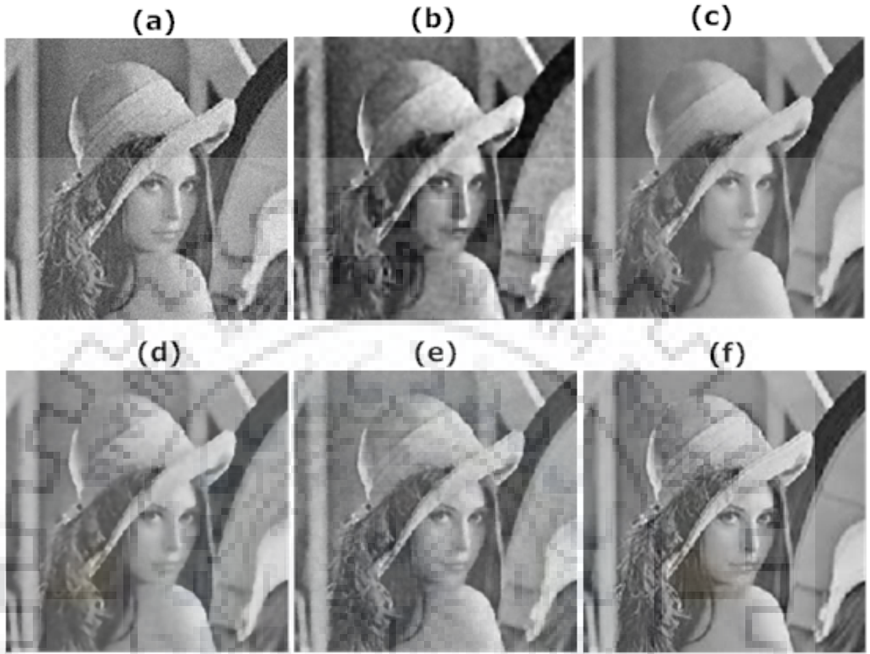
Figure 6.3: Comparison of the filtering method results for the Lena image: (a) Lena noisy image; (b) Perona and Malik based scheme [117]; (c) Guided filtering based scheme [57]; (d) Adaptive anisotropic filtering (AAF) based scheme [142]; (e) the proposed algorithm; (f) ground truth image.
