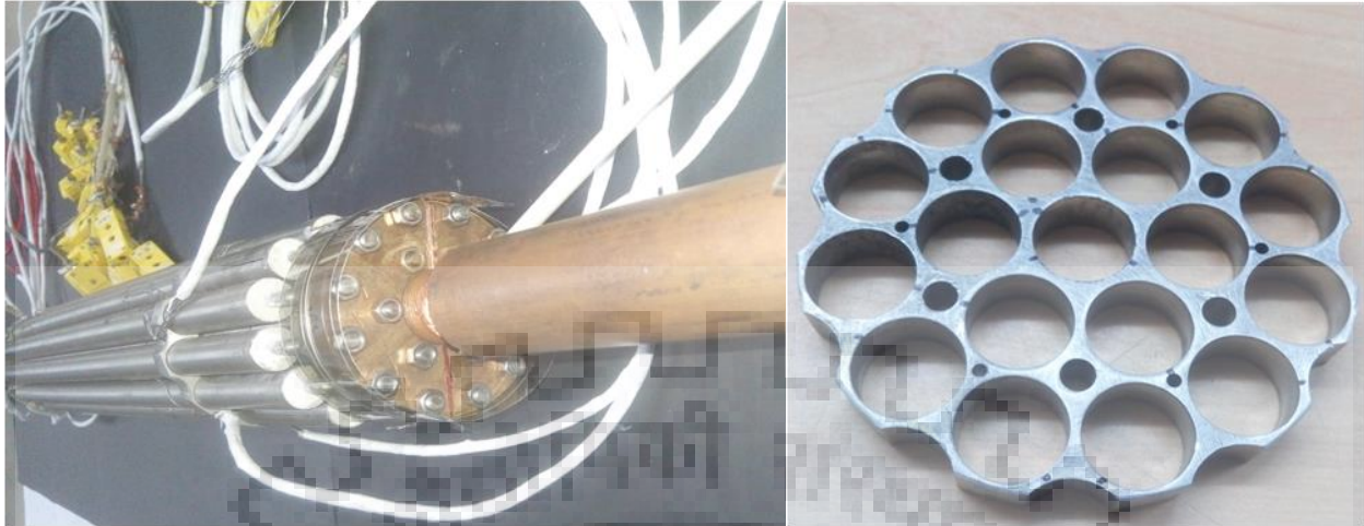
Figure 4.2. The 19 pins simulated fuel bundle and spacer.
