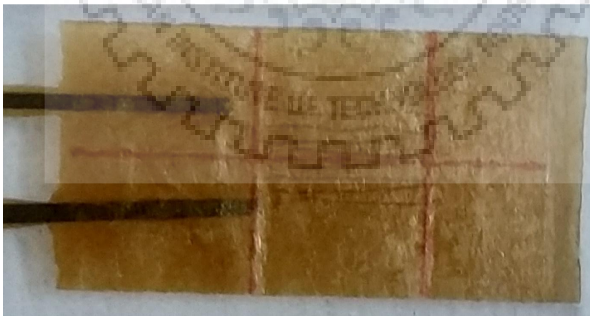
Figure 4.6 Strain gauge used for measuring strain (BKNIC-20)
